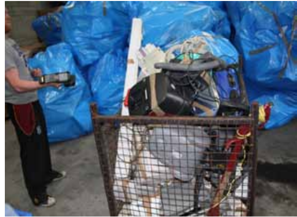
Figure 7.1. Experimental set-up with fixed-reader configuration for mixed waste electrical and electronic equipment (WEEE).
